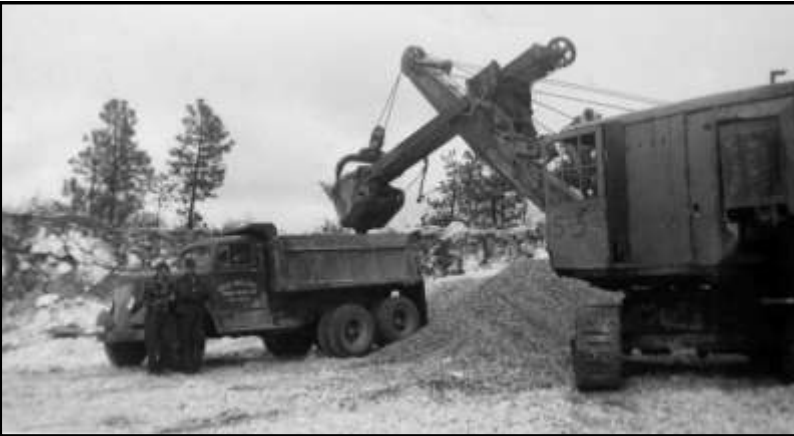
Figure 6: A Cecil Mullenix truck being loaded by a diesel shovel. What material is being loaded may be overburden as the ore was loaded from bunkers below the crusher-screening building. (Melvin Mullenix Photograph)
